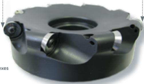
Utilizing standard Round Freedom Cutter inserts, the FCDR features totally reengineered geometry to maximize performance in Steels, Stainless, Titanium, and a wide range of High-Temp alloys. The round pocket provides increased strength and insert support. New geometry increases the shear angle resulting in increased metal removal rates and longer tool life.
