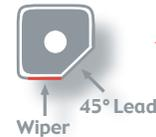
NP wipers have a single index and are installed in only one cutter pocket.
