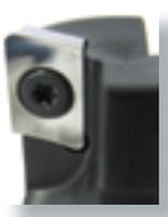
Heavy Duty, High-Velocity. The new HV3HD is the perfect mix of performance and versatility. The 100% ground and polished insert features both positive axial and radial rake, allowing the HV3HD to literally shear through the toughest materials and allowing the chip to carry away a high percentage of the generated heat. If you've been an APKT user, get ready to step up to the high-performance plate. Let's get started!
