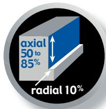
Recommendations are based upon a **radial cut depth of 10%** of the end mill's diameter and **axial cut depth of 50-85%** of the tool's LOC.
