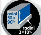
High Efficiency Milling (HEM) ratio
