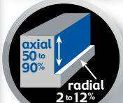
High Efficiency Milling (HEM) ratio
