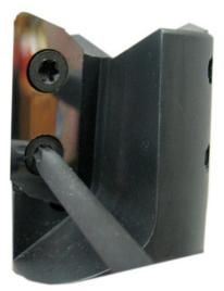
Holding the insert in place tighten the 2 bottom screw to 25 to 28 Inch LBS.
